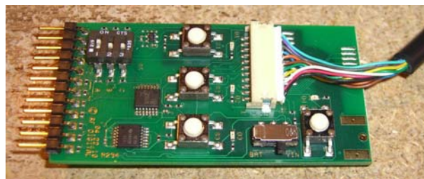
RFD21772 / RFD21773 Eval board with RFDANT cable plugged into the 11 pin connector.
